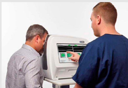
A fully-integrated OCT system
